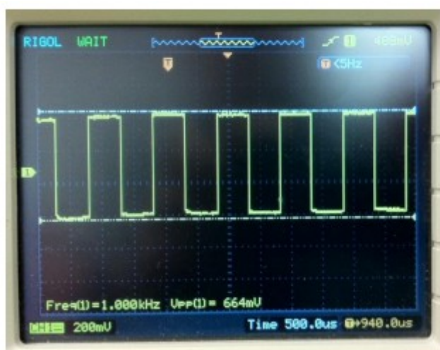
Figure 8 - 1 kHz Square Wave Response of RIAA EQ Phono Amp
