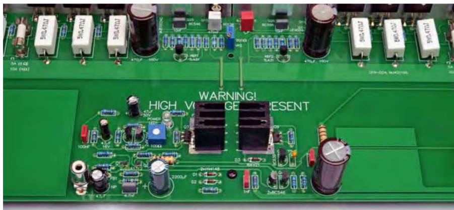
A close-up of the front-end circuitry of the 500W Amplifier Module.
