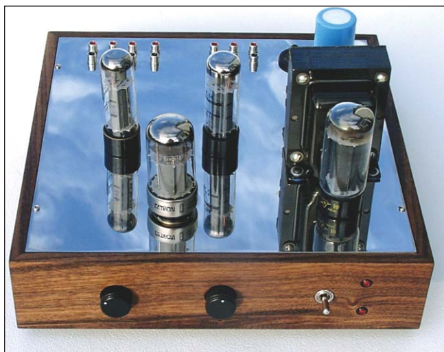
PHOTO 1: Top view of low-mu triode preamp.
