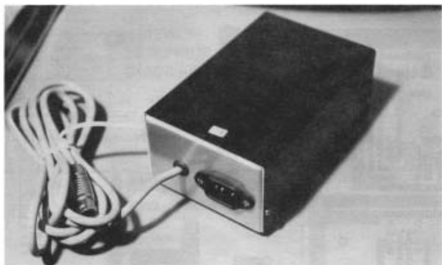
PHOTO 7: The raw DC power supply is housed in a separate enclosure with a six-pin locking connector, a modular AC power connector with its on/off switch on the front end.
