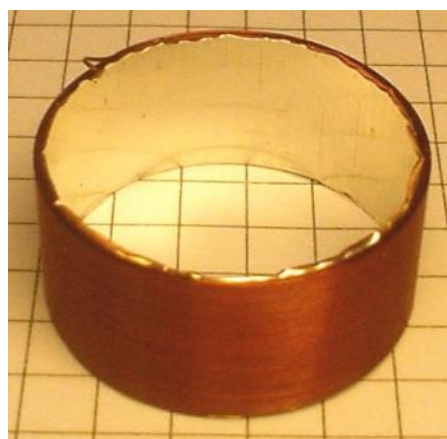
Figure 34 - The voice coil used in the woofer we are simulating
