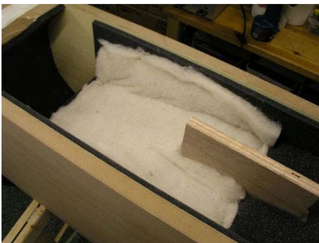
Right behind the JA8008 driver a 30 x 50 cm piece of MDM3 is folded once and fastened to the mid panel as seen on the photo.
