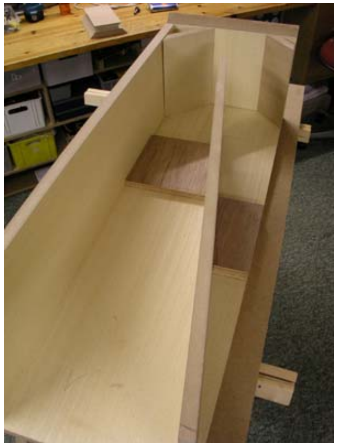
Test assembly of rear, top and side panels.
