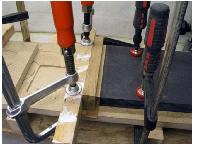
Gluing top fillet to front panel.
