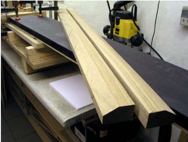
Solid 30 x 50 mm oak side bars for front panel. Chamfering is 30° at half width.
