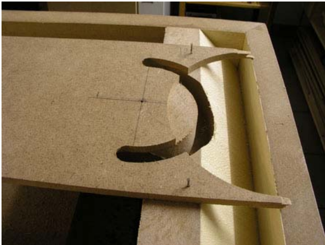
The magnet of the Audax dome needs space, thus the front reflector needs some routing.
