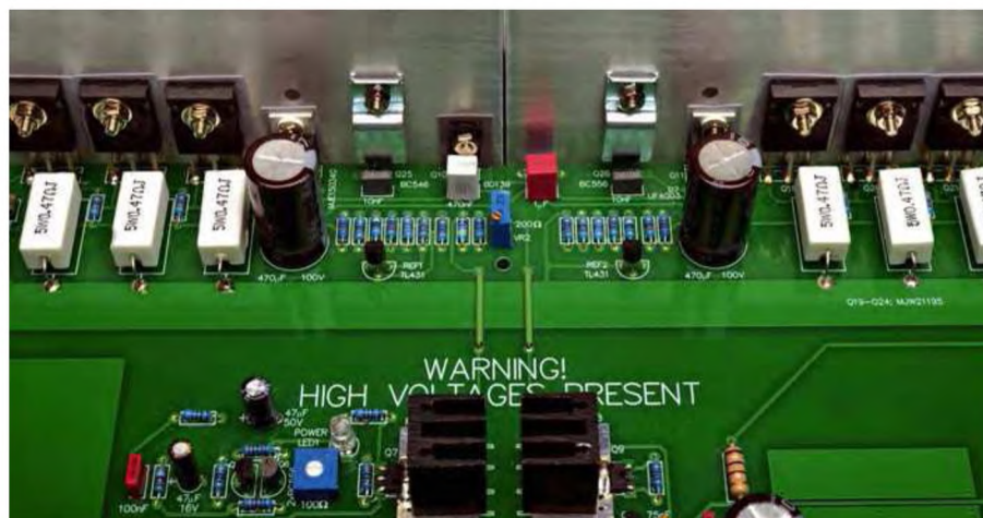
A close-up of the mounting arrangement of the transistors to the heatsink.
