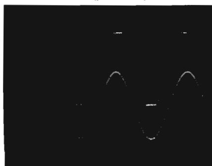
Fig. 3. Symmetrical clipping at 128W
