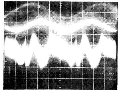
Fig 2 Distortion components 0.011% at 10 kHz.
