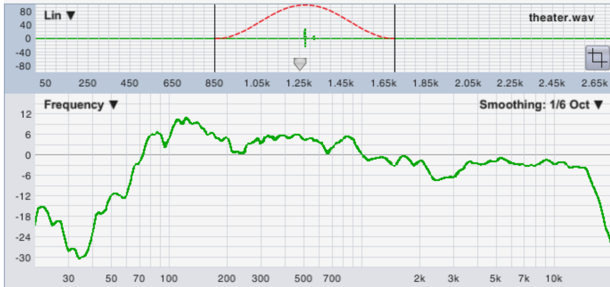
Figure 129: Moving the time 0 point and selecting a time range for display. The time range selected in the navigation pane applies to the Frequency graph as well as time domain graphs (Lin, Log or ETC). Note that Smart uses a tapered data window when transforming any subset of the full IR time range. We've drawn the outline of a Hann window in red on the navigation pane of the "result" portion of the illustration above to help visualize this.
