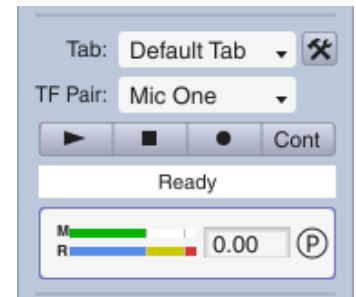
Figure 142: The measurement signal level (M) is running at a comfortable level. The reference (R) channel is clipping
