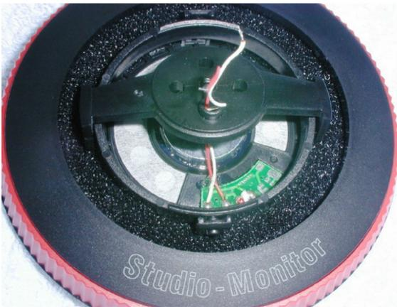
It is probably not needed to remove it and when one is handy enough the modification can be done with the 'bridge' still in place. It can be tilted to one side far enough to have good access.
