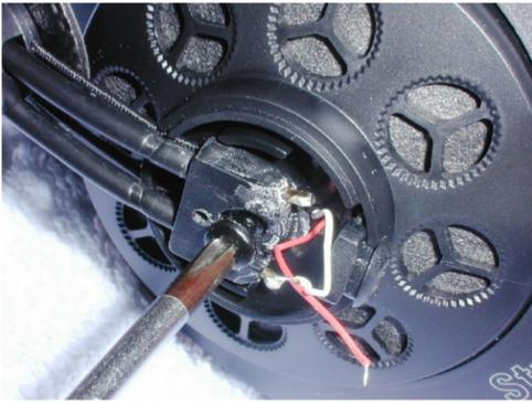
When the wires are removed the big screw must be removed. The middle part can now be removed by pulling it out. There is a paper dust filter tucked loosely in there. Once the top part is removed one ends up with the situation as shown below.
