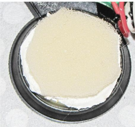
The foam used is quite open and is 5mm thick. Any open cell foam can be used. The used foam is very easy and soft to compress. The openness of the used foam (and thickness) will have an effect. Thicker foam = less bass, more dense foam = less bass.
