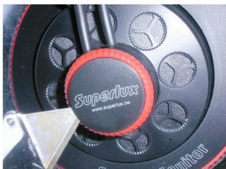
Remove the shield by sticking a utility knife under it and prying it outwards. It holds itself with 2 small pins. When the small screw is removed the cap can be removed. In this case it is the side without the cable entry.
