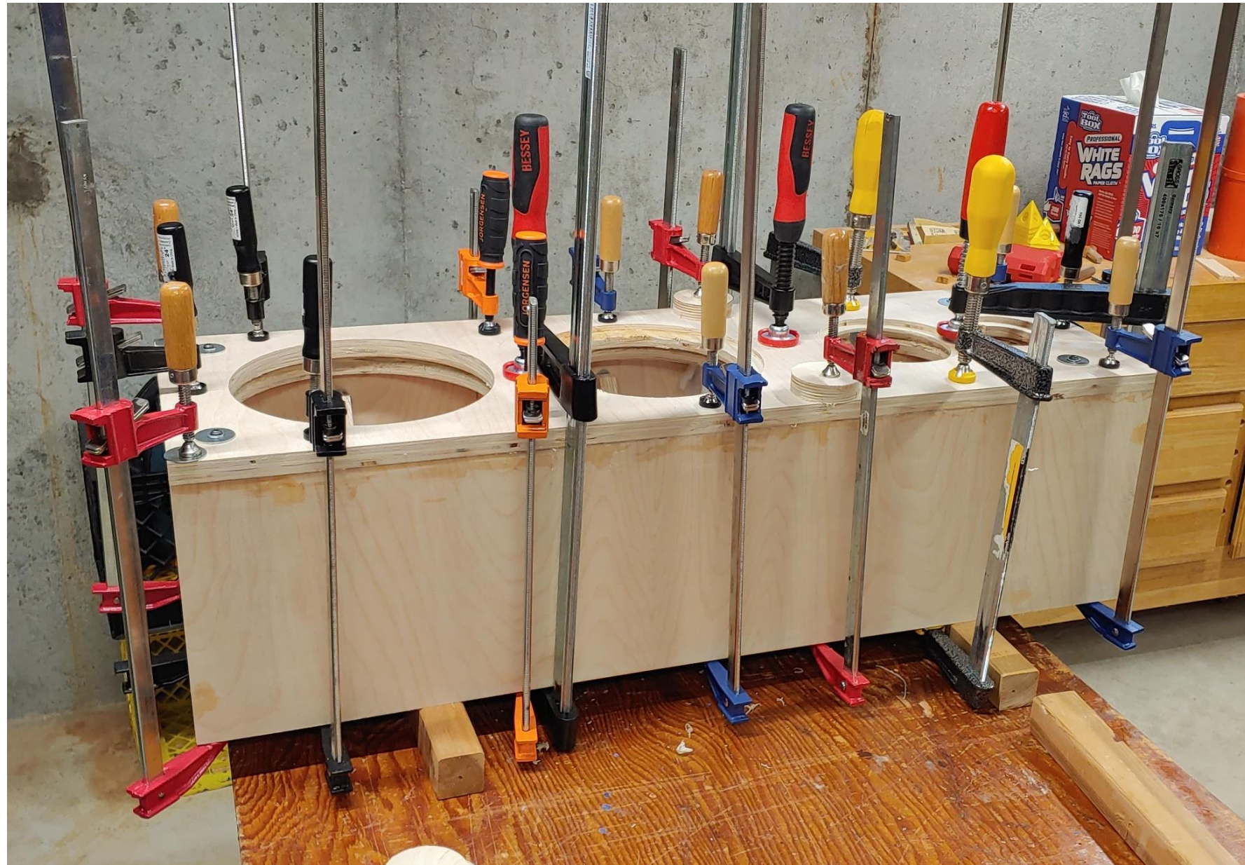
↑ Attaching the outer baffle. Total baffle thickness is 1.5" (38 mm)
