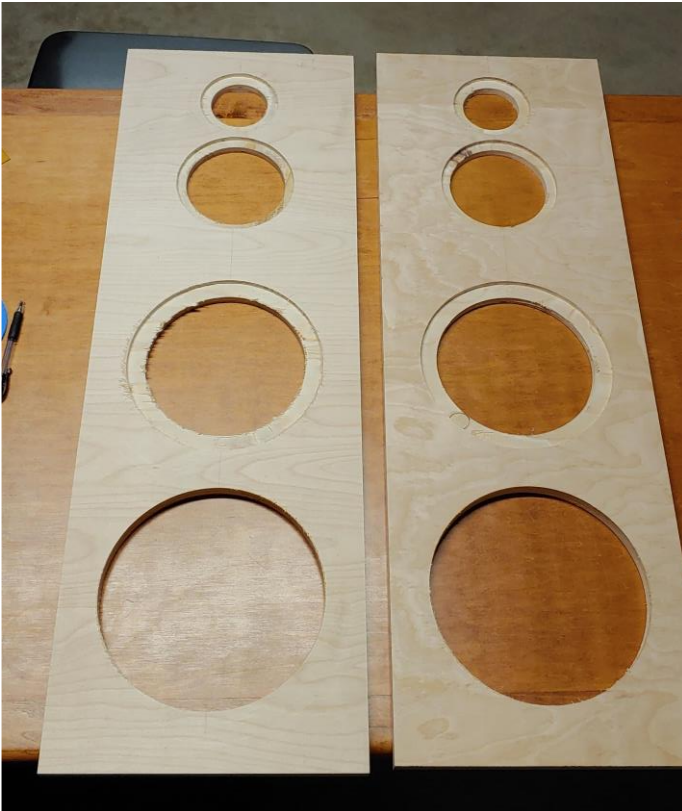
↓ Outer baffle after machining
