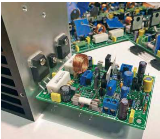
The Amplifier can be cleanly mounted to a 75mm heatsink as shown above. The SOA protection resistors are missing as we wanted to compare the performance with and without them. After which you can daisy-chain them together to form a larger system such as a six channel setup shown adjacent. This setup was mounted in a 2U rack case.
