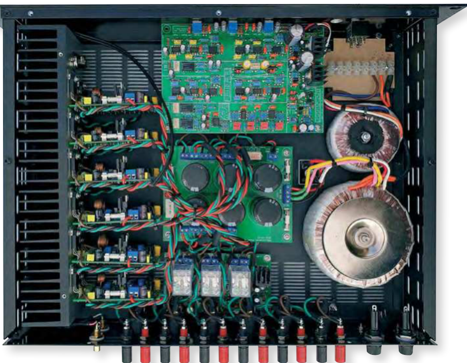
The Amplifier can be cleanly mounted to a 75mm heatsink as shown above. The SOA protection resistors are missing as we wanted to compare the performance with and without them. After which you can daisy-chain them together to form a larger system such as a six channel setup shown adjacent. This setup was mounted in a 2U rack case.
