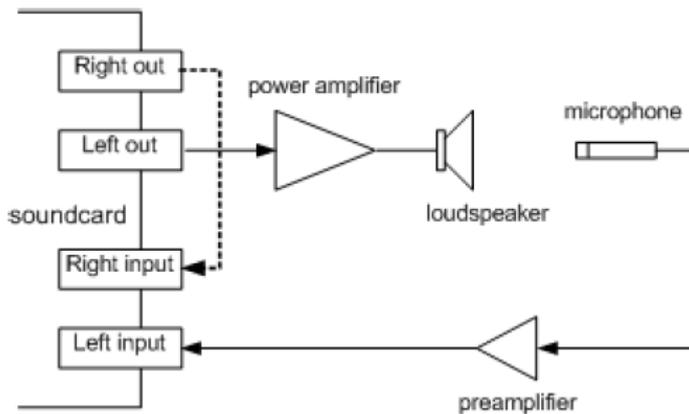
Typically microphone input of soundcard includes preamplifier and 48 V phantom power supply so external preamplifier is not needed.
