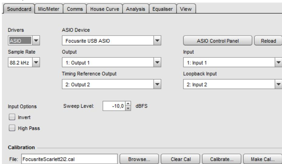
Load microphone calibration file. Example with Sonarworks XREF 20:
